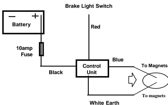
1. Connect **White** wire to (-) negative earth and direct to one side of the magnets in parallel.
