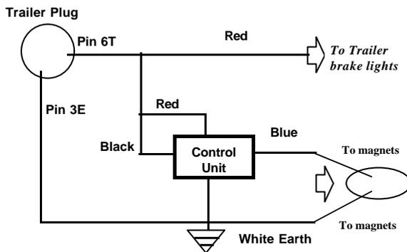
1. Connect **White** wire to (-) negative earth and direct to one side of the magnets in parallel.
